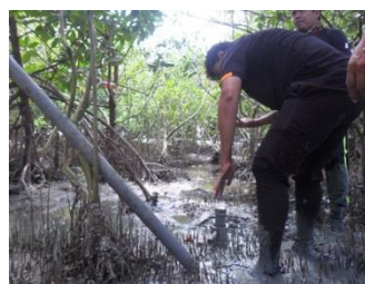
Fig. 1b: Insertion of mudflat corer into sampler with closed cap
