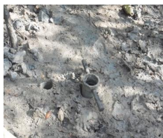
Fig.1a: Insertion of mudflat sampler
